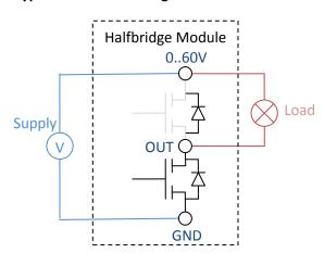
It is also possible, to leave the 0..60V connector open, but as a result the overvoltage shutdown doesn't work.
