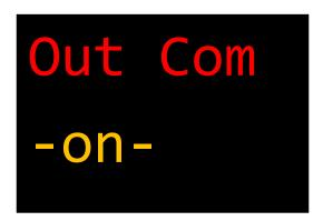
Activates/deactivates the common output. For a very fast output of the current value, the output sample frequency can be increased to 50kHz by using only one output channel.
