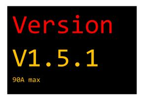
Display of the software version und the maximum continuous current of the device.
