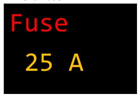
When the set threshold is exceeded, the internal electronic circuit breaker interrupts the circuit. The filter time set in the Filter menu is used as the trip time constant.
